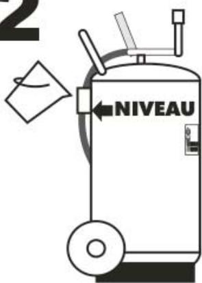
REMPLEIR LE RESERVOIR AVEC DE L'EAU PROPRE JUSQU'AU NIVEAU DE DEBORDEMENT. NE PAS PENCHER LE RESERVOIR POUR LE REMPLIR D'AVANTAGE, DANS LE CAS CONTRAIRE, L'EQUIPEMENT NE FONCTIONNERA PAS CORRECTEMENT. AJOUTER LE BACTERICIDE (ART 6800) POUR EVITER LA FORMATION D'ALGUES.
